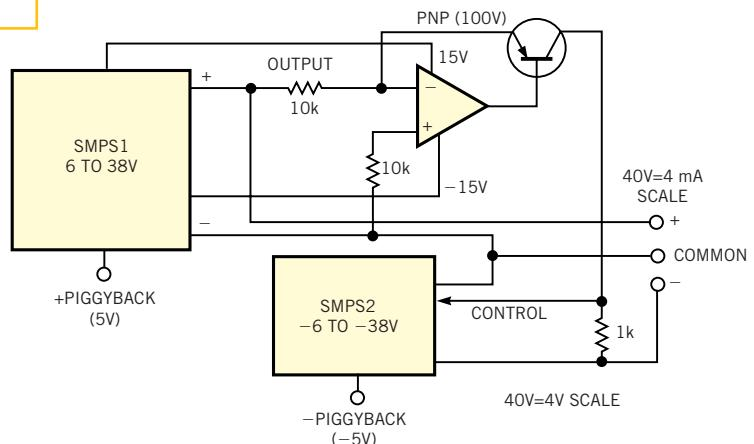
The switch-mode power supplies track each other with opposite-polarity outputs.
