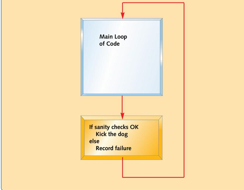
will be no false watchdog resets. On a medical ventilator, 10 seconds would have been far too long to leave the patient unassisted, but if the device can recover within a second then the failure will have minimal impact, so a choice of a 500ms timeout might be appropriate. When making such calculations be sure to include the time taken for the device to start up as well as the timeout time of the watchdog itself.
