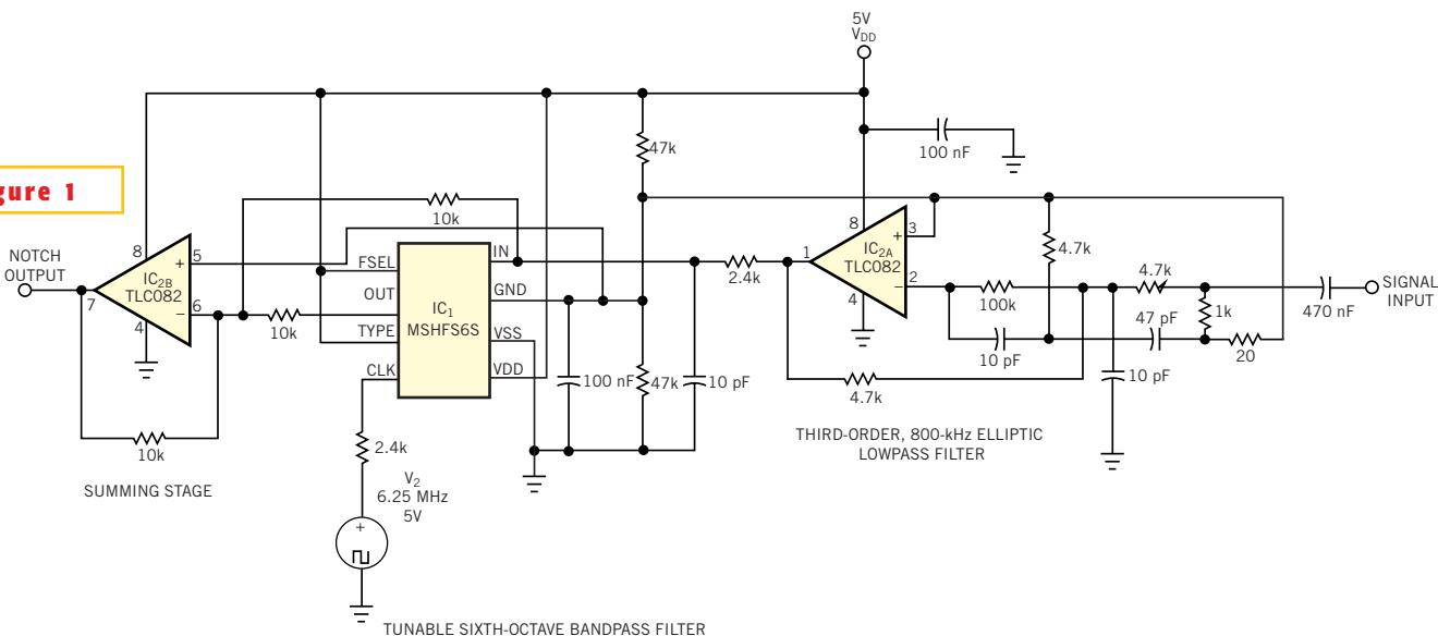
An op amp and a switched-capacitor filter combine to form a highly selective notch filter.
