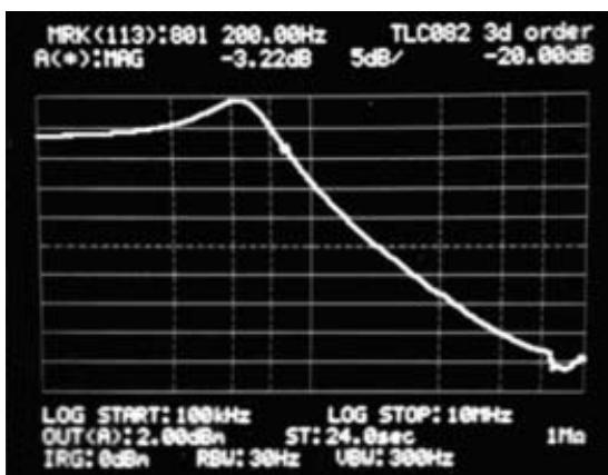
Figure 2 This plot is the frequency response of the third-order lowpass-filter stage.
