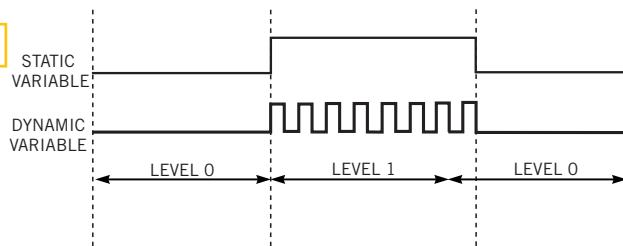
You can improve the reliability of an electronic-control output by using an oscillating, instead of steady-state, signal to represent a logic-high state.
