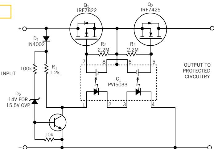
This polarity-protection circuit incurs lower forward-voltage drop than the best Schottky diodes.
