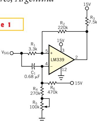
**By presenting the noise signal to both inputs of the comparator, this circuit can compare the dc levels of the signal and the reference.**
