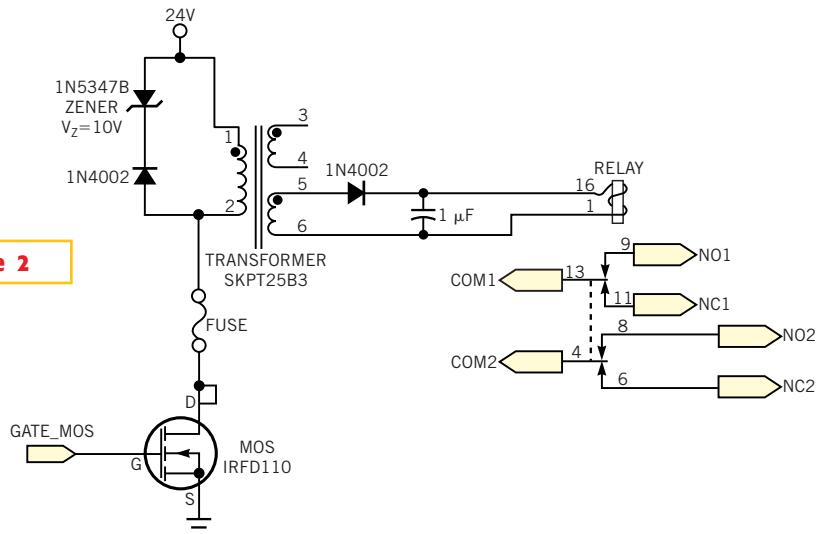
A "dynamic-variable" signal drives the output relay in this circuit.
