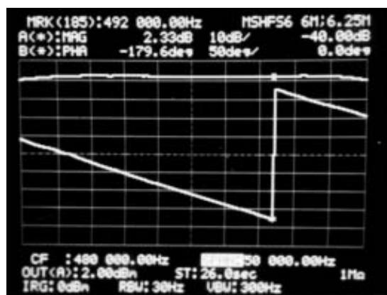
Figure 3 This Bode plot represents the passband of the MSHFS6 filter.
