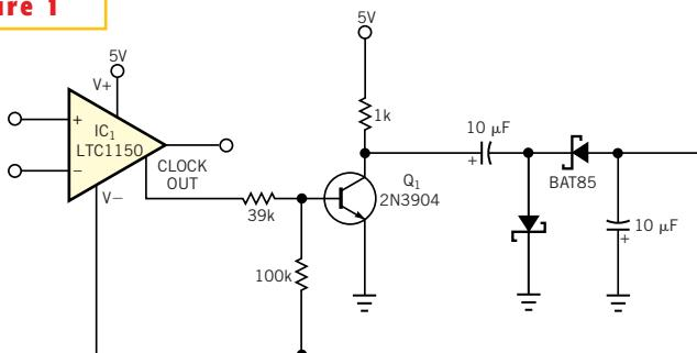
This configuration uses bootstrapping to allow a single-rail op amp to operate at 0V output.
